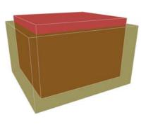
Fig. 1. Conservation of authentic facade of the building and change of its interior structure. Source: ill. S. Hanets
